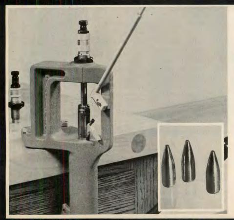
Pacific Tool Company (A division of Hornady), Dept. SOF, Box 2048, Grand Island, NE 68801, exhibited their new Positive Priming System. The automatic primer eliminates individual primer handling and reduces priming cycle time. One cycle moves the primer arm under the automatic primer feed, picks up a primer, moves it into the ram cavity and up into the die where it is seated. The new primer system comes with the new 0-7 reloading press and costs \$59.95.
